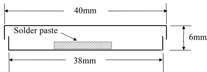
After removing grease from the both copper plate A and B with acetone, soak them in 5% sulfuric acid for 1 minute and in ammonium persulfate solution (solution which contains 25% of ammonium persulfate in 0.5% of sulfuric acid) in 1 minute to etch the surface uniformly. After washing them with running water, soak in 5% sulfuric acid for 1 minute and rinse thoroughly with running tap water and demineralized water. Then, finally, rinse them with acetone and dry.
