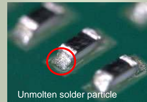
Sample A After 8hrs rolling
